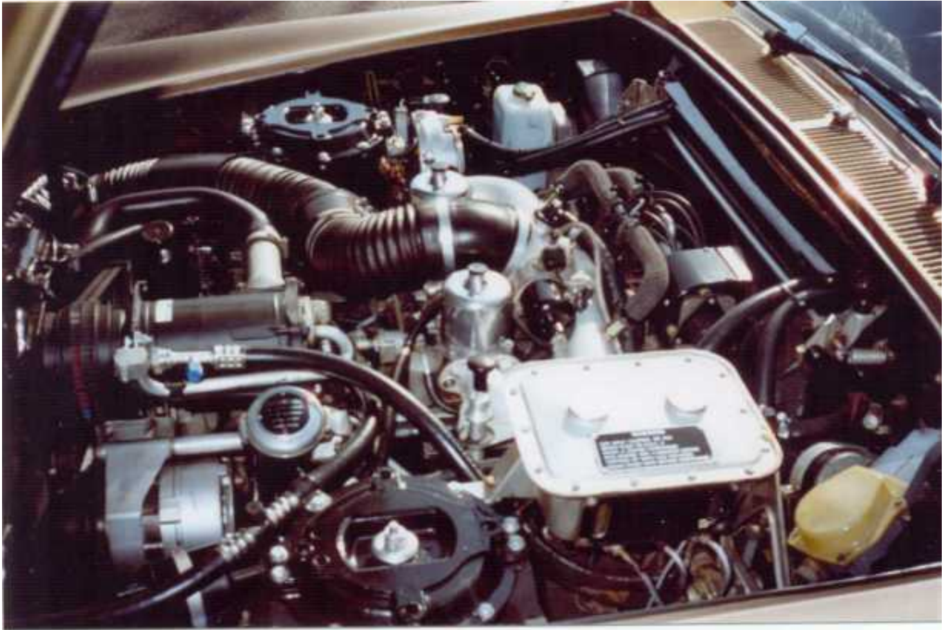
Another view. Snuggled behind the suspension tower is the converter (Driver's side)
